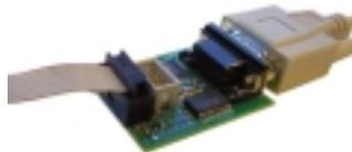
**Figure 3-4.** AVRISP with 6-pin ISP Connector
