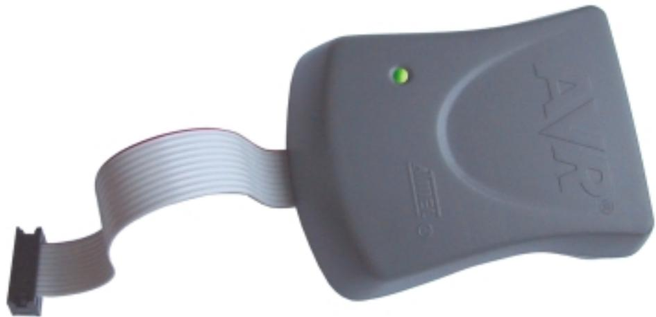
The AVR<sup>®</sup> In-System Programmer (AVRISP) from Atmel<sup>®</sup> is a professional low-cost In-System Programmer covering all AVR 8-bit RISC Microcontrollers. The programmer connects to a PC through a standard RS-232 serial interface and draws the necessary power from the target board eliminating the need for an additional power supply. AVR Studio<sup>®</sup> is used as front-end software, giving you a highly-integrated development solution.
